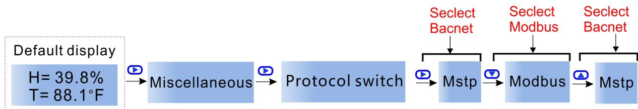
Or you can check the Bacnet Register List, No.9: Protocol switch. 0 = MODBUS, 1=MSTP.
