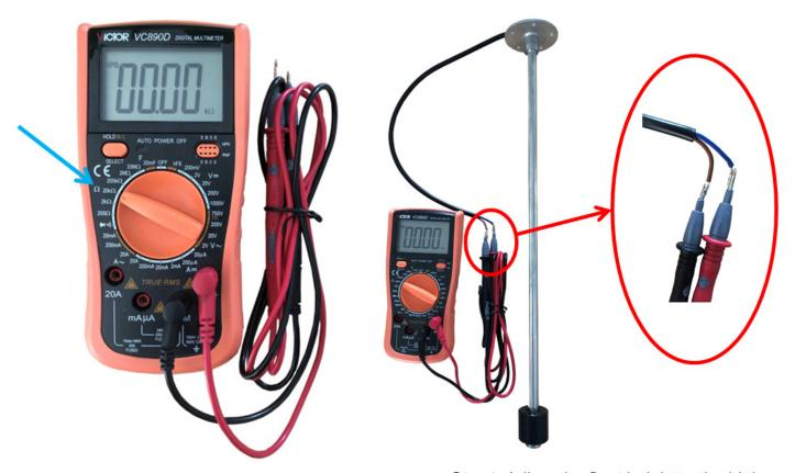
Step3: Set the float height to the lowest read resistance Step4: Adjust the float height to the high-value, as shown est read resistance value, as shown
