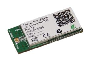
This module can achieve transparent data transmission between many devices, and it can form a MESH network. This device has the characteristics of small volume, ultra-low power consumption and low-cost. It can be either as an independent data transmission termination or be easily embedded into a variety of products to form a short-range wireless data transmission solution.
