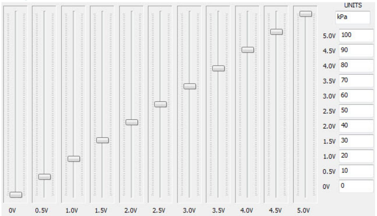
As an example of a custom sensor, here we have built up a table for a custom sensor operating from 0 to 5V over the range of 0-100psi.
