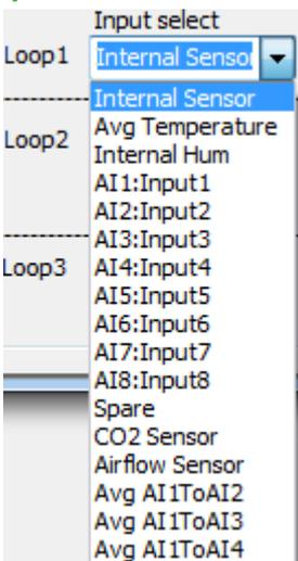
For the PID feedback you can select from many options such as the average of some sensors, any of the 8 external sensors or the internal humidity or CO2 sensor if it has one.
